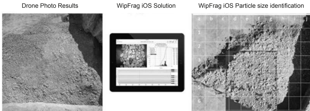
Figure 2. Fragmentation Analysis using WipFrag w/GIS
